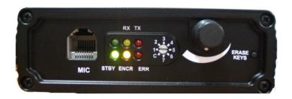
Figure 6: Encryption Mode Indications
